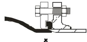
Flange bolts must not be over tightened, bolts should be tightened gradually and evenly and in a crosswise manner. Bolts should be positioned so that the bolt head is nearest the bellows to prevent the bolt damaging the bellow in service. Tightness of bolts should be checked approximately seven days after installation.
