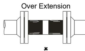
Only the correct mating flanges should be used. They should be the same size and drilling and have a similar sealing face as that of the rubber bellows. They must be clean and free from any debris, sharp edges etc. to prevent damage occurring to the sealing face of the bellows. For mating flanges with a different sealing face diameter a composite gasket should be used to prevent any sharp edges cutting into the rubber sealing face.
