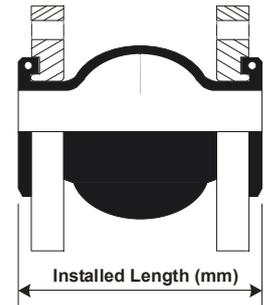
**Installation** Rubber bellows should be installed at their neutral (supplied) length. Confirm that the gap left between the mating flanges in the pipework corresponds exactly with the neutral (supplied) length of the rubber bellows. Pipework should be true and straight. Any adjustments should be made to the pipework before the rubber bellows are fitted. See appropriate Stourflex data sheets for the installation length of the rubber bellows being installed.
