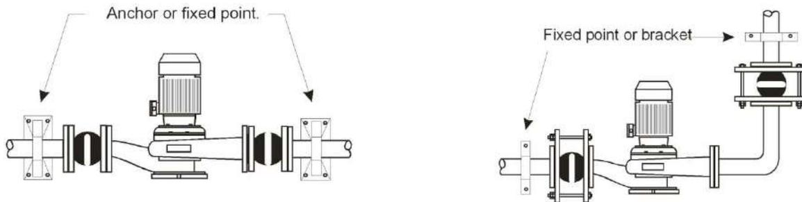
Rubber bellows will exert a pressure thrust in service and must be anchored to protect adjacent pipework and equipment. Rubber bellows will extend under pressure and must be anchored to prevent this happening.
